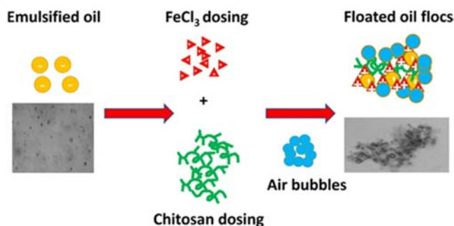
Figure 7.4 The hybridized coagulant/flocculant system, using ferric chloride as coagulant and chitosan as biodegradable flocculant, was added for DAF process. Ferric chloride and chitosan were added during the rapid and slow mixing steps, respectively. The addition of dissolved air at the end of the slow mixing step induces buoyancy as the air bubbles attach to the oil flocs to form floc-bubble aggregates and float to the top of the jar. This accelerates the clarification of the water [49].
